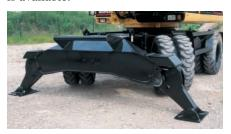
**Outriggers.** The pin-on design allows the outriggers to be mounted on the front and/or rear for maximum operating stability when digging or lifting and are individually controlled for leveling on slopes.
