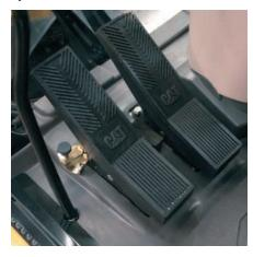
**Foot Pedals.** Two-way pedals for travel and auxiliary circuits give more floor space and reduce the need to change positions. The foot pedal for auxiliary high-pressure circuit can now be locked in the off position and is used as a footrest for greater operator comfort.
