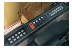
**Control Convenience.** Each control is placed within easy reach of the operator. Joysticks control the implement functions, steer the machine while in first gear and activate the adjustable hydraulic sensitivity. The soft switch panel controls the oscillating axle, power control settings, parking brake, automatic engine speed control, and other hydraulic functions.
