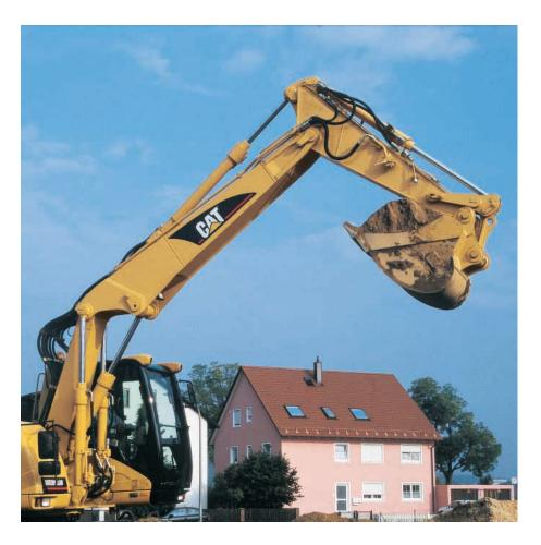
**Design.** Booms and sticks are welded, box section structures with thick, multi-plate fabrications in high stress areas and are built for performance and long service life.
