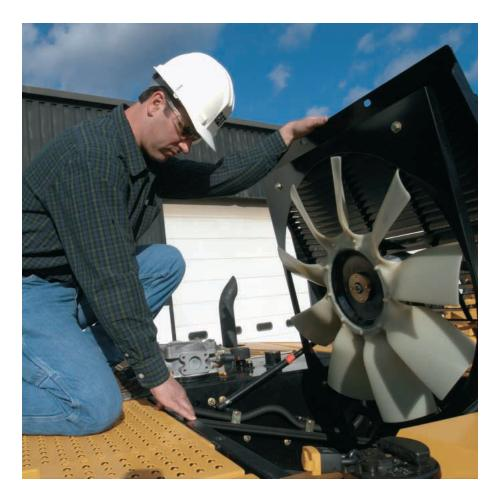
**Easy Access.** Gull-wing doors, with pneumatically-assisted lift cylinders, effortlessly lift up for exceptional access to the engine and all service points. An additional toolbox located under the step leading to the upper platform offers clean, dry storage for the operator.
