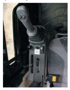
**Consoles.** Designed for simplicity and functionality. The left side console is tiltable for excellent access to the cab. Dozer blade and/or outrigger controls as well as the radio-off switch are located on the left console.
