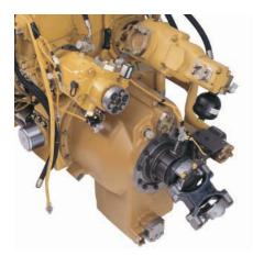
**Torque Divider.** A single-stage torque converter with output torque divider sends 75 percent of engine torque through the converter and 25 percent through a direct drive shaft for greater driveline efficiency and higher torque multiplication. The torque converter shields the driveline from sudden torque shocks and vibration.
