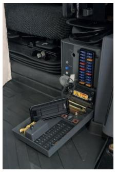
**Fuse Panel and Diagnostic Access.** The new compartment features a single location fuse panel that includes a diagnostic port for the Cat ET to connect for rapid machine diagnostics.
