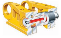
**Positive Pin Retention (PPR) Sealed and Lubricated Track.** Designed for high-impact and high load applications. The PPR exclusive Caterpillar design locks the link to the pin.
