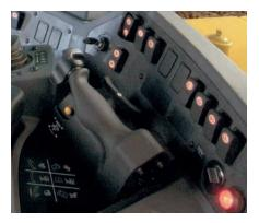
**Ripper Control Lever.** A rigidly mounted handgrip provides firm support for the operator even when ripping in the roughest terrain. The low effort thumb lever controls raising and lowering. The finger lever controls shank-in and shank-out positioning. The thumb button automatically raises the ripper.
