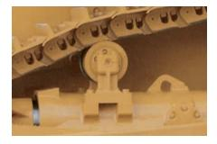
**Integrated Carrier Roller Mount.** The carrier roller mount is cast into the track roller frame making it easier to add the optional carrier roller in the field, if conditions require it.
