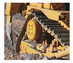
**Suspended Undercarriage Design.** Suspended undercarriage design absorbs impact loads, to reduce the shock loads transferred to the undercarriage, by up to 50 percent in uneven terrain.
