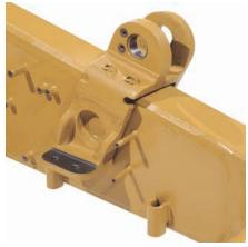
**Engine and Radiator Guard Mount.** The new fabricated common front engine and rear radiator mount feature heavy castings.
