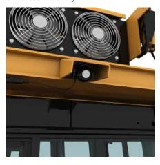
**Rear Vision Camera.** An attachment WAVS rear vision camera is available to provide additional visibility to the standard mirrors.
