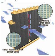
Radiator (AMOCS). The AMOCS radiator utilizes an exclusive two pass cooling system and increased cooling surface area to provide significantly more cooling capacity than conventional systems. A trash core radiator is available with six fins per inch, replacing the standard nine fins per inch.
