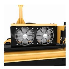
**ROPS-mounted Air Conditioner Condenser and Fans.** The ROPS-mounted air conditioner and fans are relocated from the engine compartment to the ROPS.
