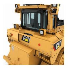
Hydraulic and Fuel Tank guard. The hydraulic and fuel guard helps protect implement hydraulic oil tank, battery box and fuel tank.
