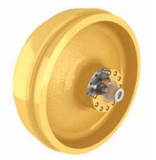
**Idler Seal Guards.** The idler seal guards help keep wire, fishing line, strapping, etc., from wrapping around and damaging the Duo-Cone seals.
