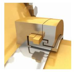
**Seal Guard Design.** This design offers superior protection to the seal. Debris would have to make four 90° turns, penetrate the packing material, and then make two additional 90° turns.
