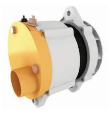
**High-capacity Alternator.** The high-capacity 95-amp alternator provides additional power required for electrical accessories such as supplemental lights and communications and entertainment radios. The ducting helps prevent debris from entering into the alternator.
