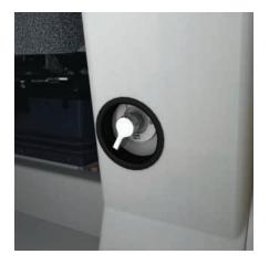
Remote Disconnect. Located in the cab, the remote disconnect switch is in series with the standard machine disconnect. The switch, located on the left side of the operator seat at knee level, allows the operator to access the disconnect switch quickly.
