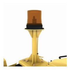
**Beacon Light.** A heavy-duty Federal Signal Pulsator 551 single flash (5 joules) strobe beacon unit is weather sealed and water resistant with the power supply encased in gel. The beacon is wired directly and can only be turned off by the disconnect switch. Extends above the highest part of the machine for enhanced visibility.
