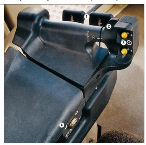
**Automatic Shifting** features easier upshifts and downshifts which can increase operator productivity, reduce fatigue, and shorten cycle times.
