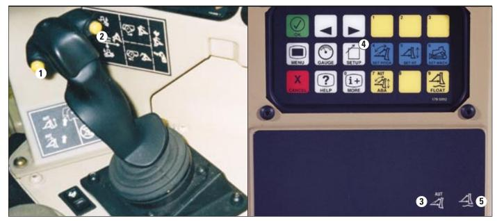
**Automated Blade Assist (ABA)** is a semi-automatic dozer control function that increases efficiency and reduces operator workload by automating some of the more common blade functions. The ABA system for Carrydozer tractors consists of AutoPitch, AutoSpread, and Auto Return.
