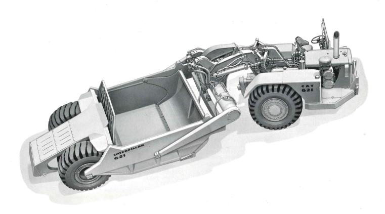
**Positive-Action Scraper** is hydraulically controlled for positive cutting edge penetration, apron closure and material ejection.
